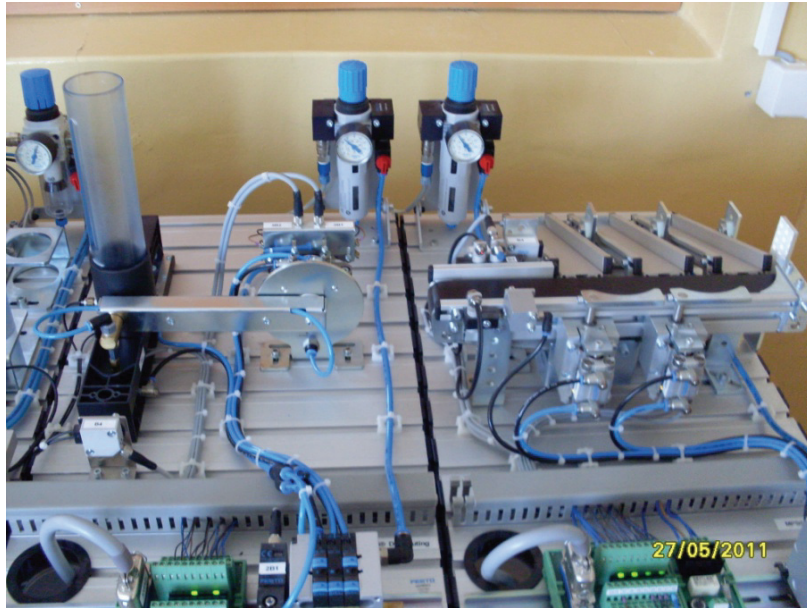
Fig. 3. Distributing and sorting station
