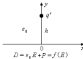
Fig. 1. Uniform line charge over non-linear infinite media.
