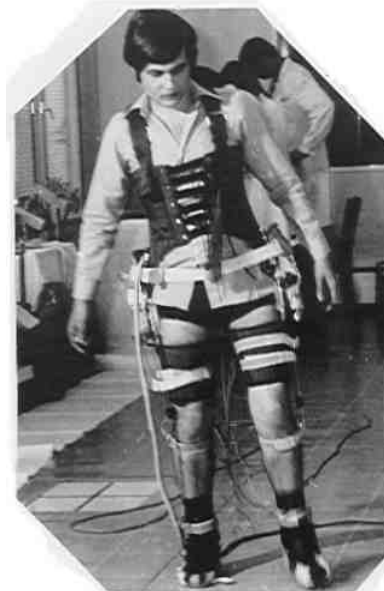
Fig. 4. Belgrade active exoskeleton exhibited in the Polytechnical Museum in Moscow as an item of the basic fund of objects
