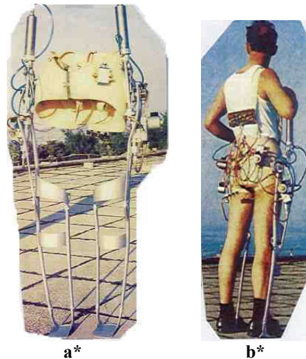
Fig. 2. a* and b* First in the world walking active exoskeleton, pneumatically powered and partly kinematically programmed, for producing near-anthropomorphic gait. Made in 1969 at the Mihajlo Pupin Institute, a predecessor of more complex exoskeletons devices for severely handicapped persons.
