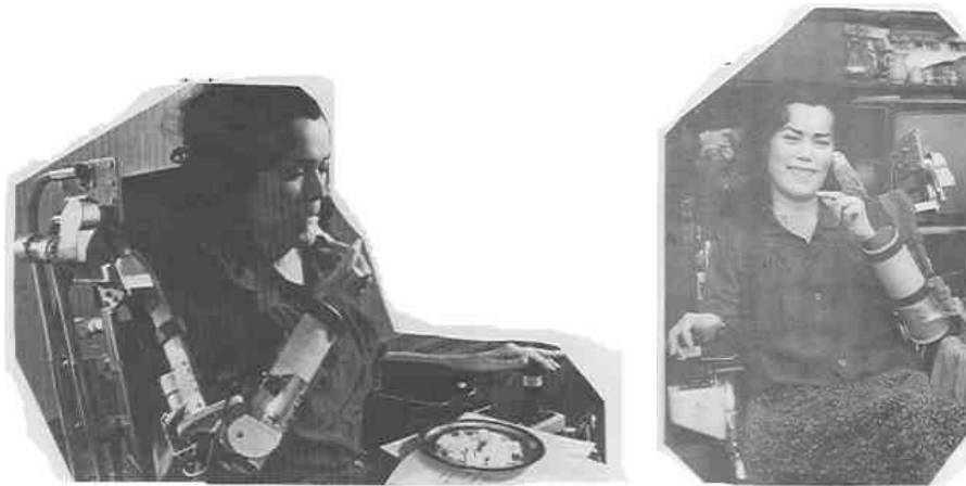
Fig. 6. Successfully developed active arm orthosis for rehabilitation of advanced cases of dystrophy and similar diseases. Controlled by means of a joystick. Made in Mihajlo Pupin Institute in 1982.
