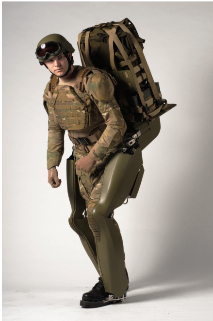
Fig. 12. "BLEEX" [8] Project is financed by DARPA It can load up to 32 kg. Man has feeling like 2 kg is on his back. The aim is to improve load up to 60 kg with feeling like 4 kg.
