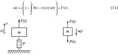
Fig.1 a) a simple oscillator with hereditary element P b) a scheme of the forces acting on the oscillator mass.
