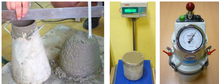
Fig. 3 Testing the fresh concrete properties: Slump test (left), Density test (middle), Air content test (right)
