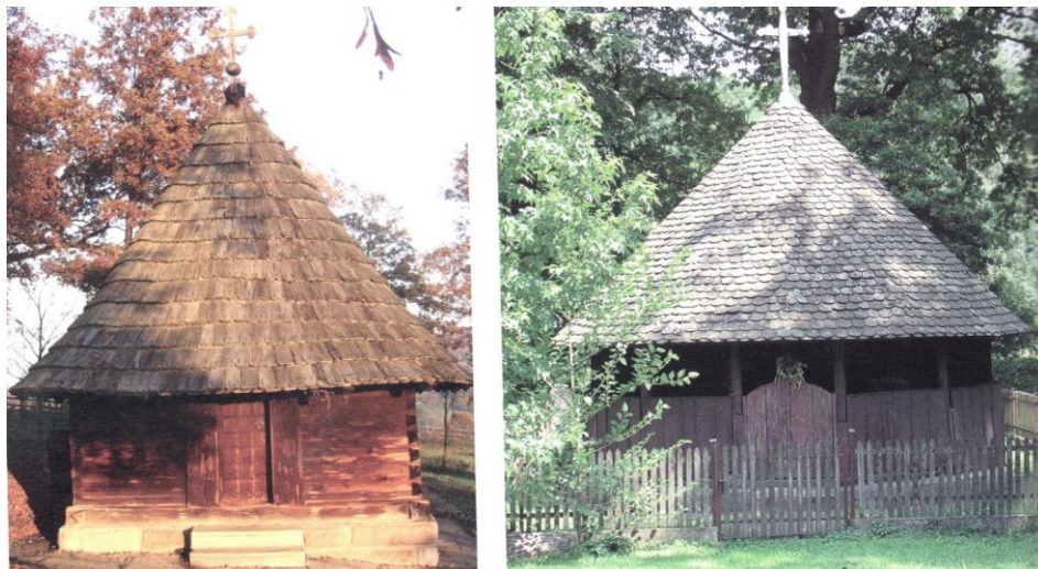
Fig. 1. Log churches – constructed with no use of connectors
