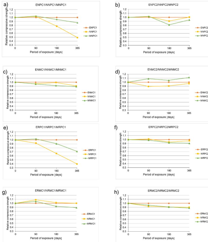
**Fig. 1** Changes of compressive strength of concretes exposed to sulfate solutions in relation to corresponding strength of control specimens (a – NA, CEM I, w/c=0.55, b – NA, CEM I, w/c=0.38, c – NA, CEM III, w/c=0.55, d – NA, CEM III, w/c=0.38, e – RCA, CEM I, w/c=0.55, f – RCA, CEM I, w/c=0.38, g – RCA, CEM III, w/c=0.55, h – RCA, CEM III, w/c=0.38)
