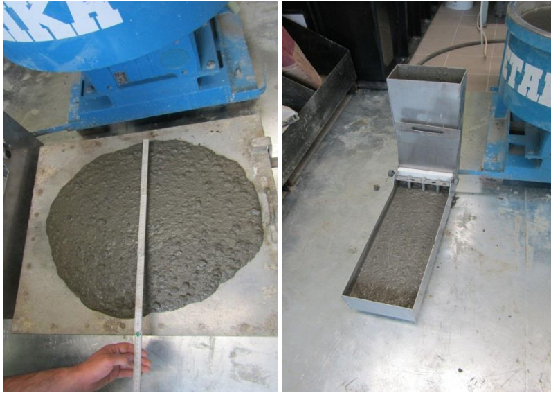
Fig. 3 Slump flow test and L – box test
