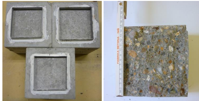
Fig. 4 Appearance of the specimens after the tests of resistance to simultaneous action of frost and salt (left) and the appearance of the specimen after water permeability test
