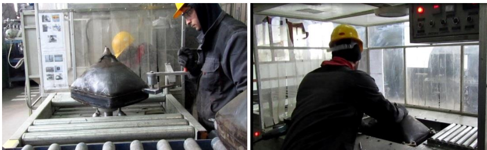
Fig. 2 System for lining out and separation of integral parts of a monitor using hot wire.
