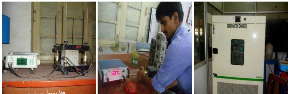
(a) Electrical Resistivity Meter (b) Ultrasonic Pulse Velocity Test (c) Carbonation Chamber
