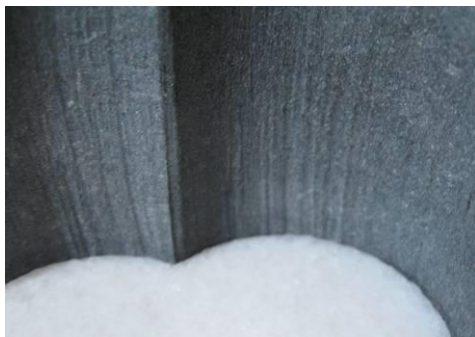
Fig. 3 Cut surface generated by abrasive water jet cutting of granite
