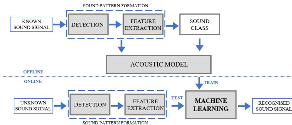
**Fig. 1** Architecture of system for detection and classification of sound events
