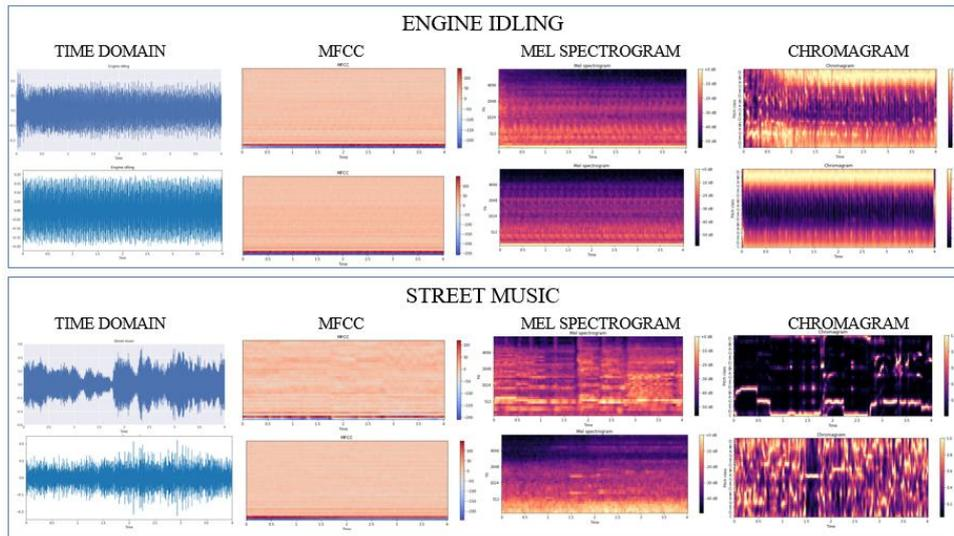
**Fig. 6** Visual representation of the used audio parameters of the sound events ‘engine idling’ and ‘street music’
