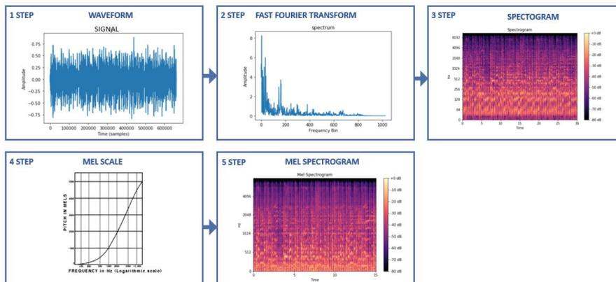
**Fig. 3** MEL Spectrogram feature extraction steps
