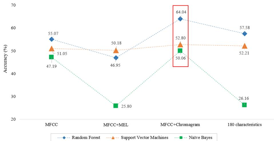
**Fig. 5** Accuracy results using different audio parameters and ML algorithms
