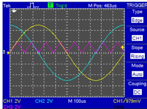
Fig. 5 Sine (CH1), cosine (CH2) and quasi-linear signal (CH3) displayed using Tektronix oscilloscope
