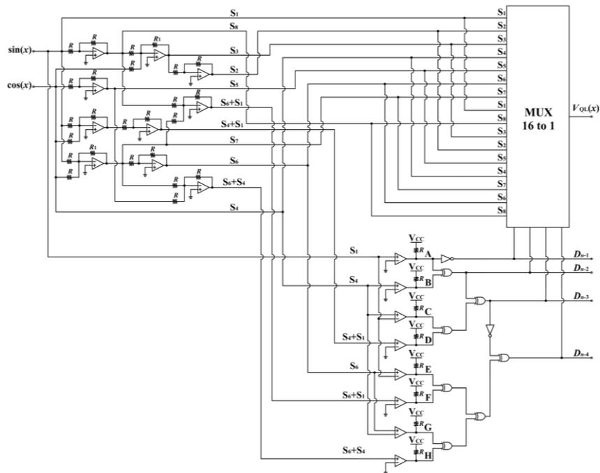
Fig. 1 A 4-bit mixed analog-digital circuit
