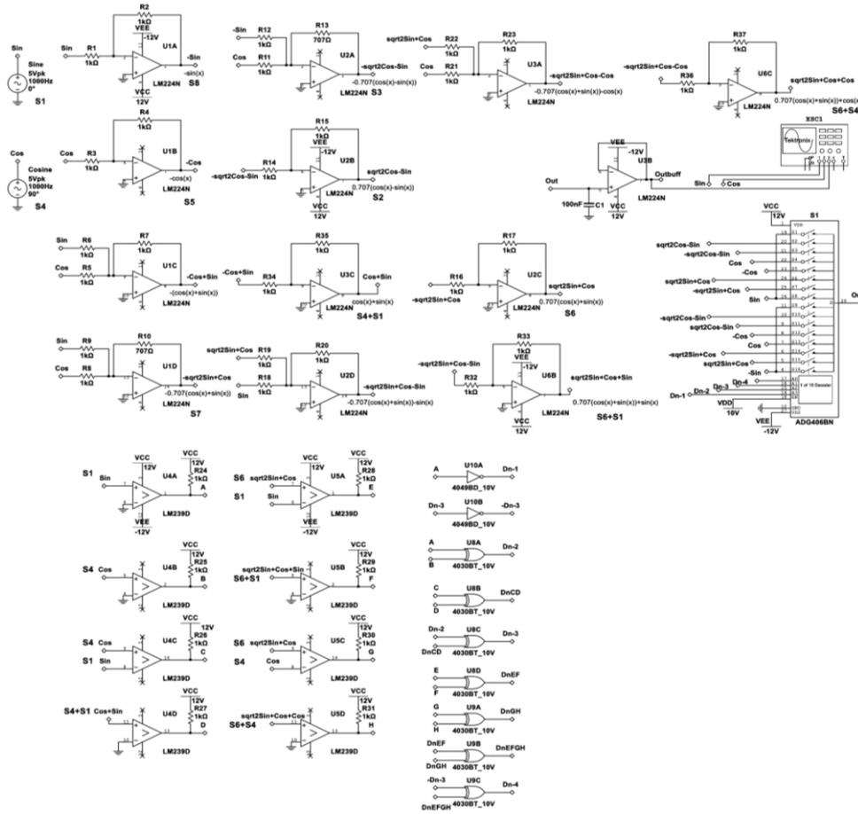
Fig. 4 A Multisim simulation of the 4-bit mixed analog-digital circuit
