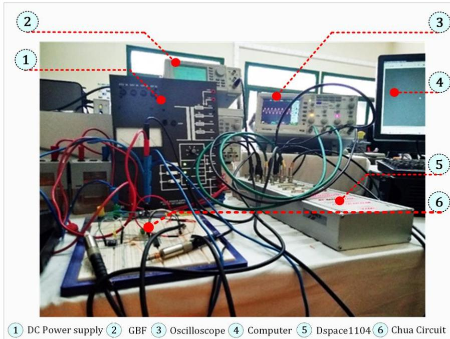
**Fig. 5** Experimental setup
