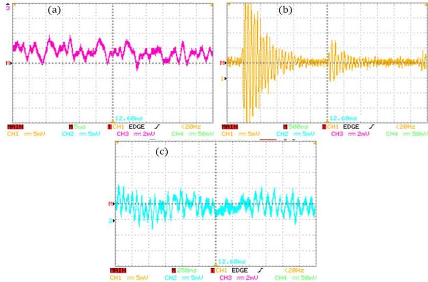
**Fig. 6** Experimental results in open loop: (a) current Inductor  $I_L$  (b) voltage capacitor  $V_{C_1}$  (c) voltage capacitor  $V_{C_2}$
