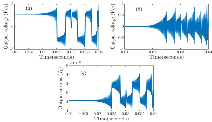
**Fig. 3** Simulation results in open loop using proteus platform: (a) voltage capacitor  $V_{C1}$ , (b) voltage capacitor  $V_{C2}$ , (c) current Inductor  $I_L$
