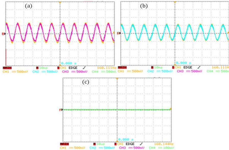
**Fig. 7** Experimental time response of the state variables in closed loop with: (a) voltage capacitor  $V_{C_1}$ , (b) voltage capacitor  $V_{C_2}$ , (c) Time responses of the tracking errors
