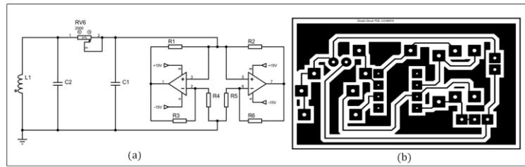
**Fig. 2** Chua's circuit prototype: (a) schematic under Proteus, (b) PCB design
