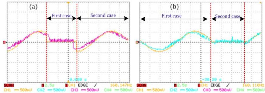
**Fig. 8** Time response of the state's variable with different reference (a) capacitor voltage  $V_{c1}$ , (b) capacitor voltage  $V_{c2}$
