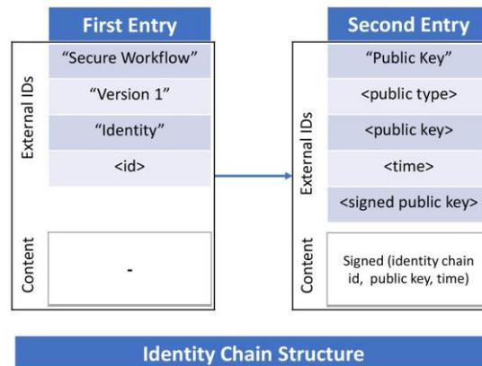
**Fig. 2** Identity Chain structure of the proposed system.
