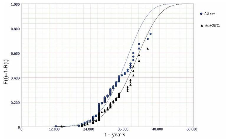
**Fig. 3** Weibull unreliability distribution for CBs on underground feeders
