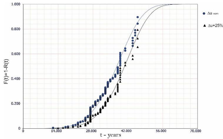
**Fig. 4** Weibull unreliability distribution for CBs on 10 kV overhead feeders
