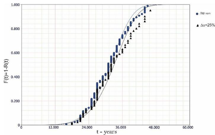
**Fig. 5** Weibull unreliability distribution for CBs on 35 kV overhead feeders
