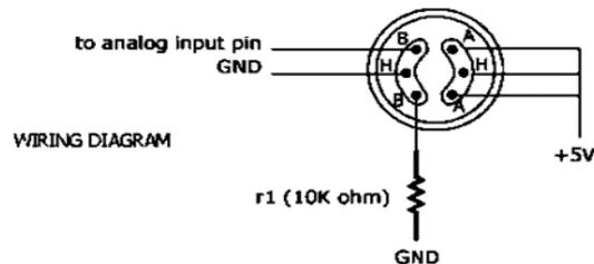
Fig. 4 MQ-6 gas sensor equivalent circuit schematic.
