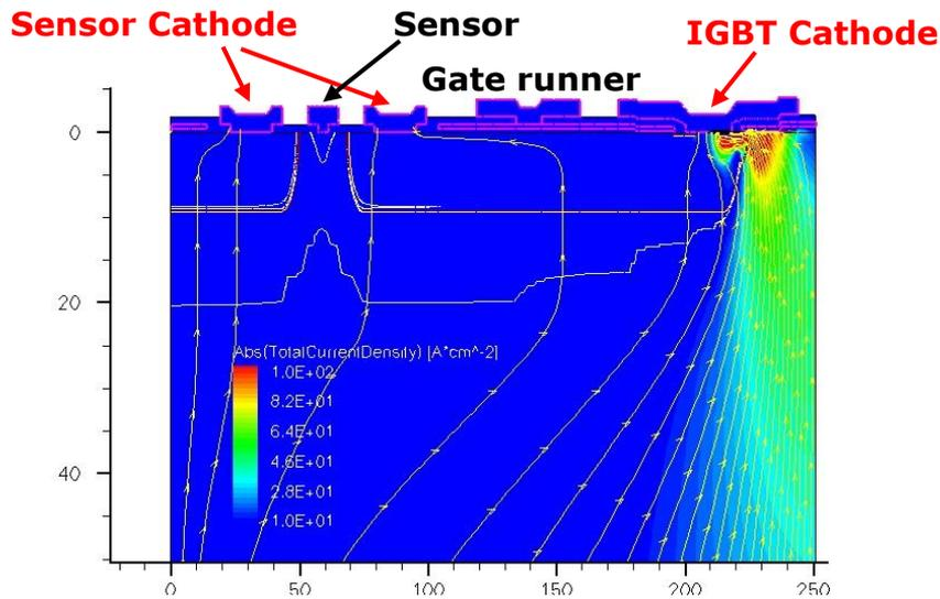
**Fig. 4** Current flowlines at a gate bias of 15 V in the last IGBT core cell and the first anode voltage sensor strip
