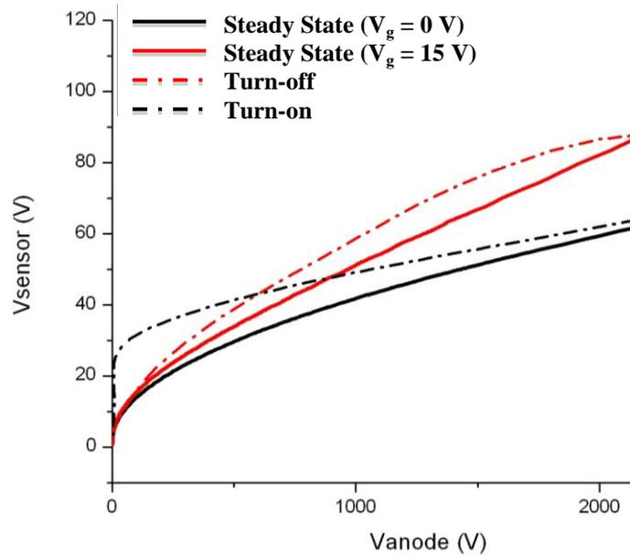
**Fig. 8** Steady and transient simulation of the anode voltage sensor level as a function of the applied anode voltage
