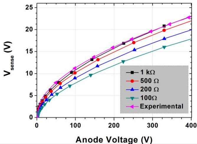
Fig. 6 Simulated and experimental evolution of the voltage sensor value as a function of the resistive load of the control electronics
