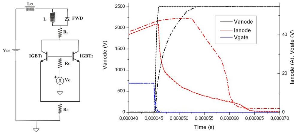
**Fig. 7** Test circuit for the inverter switching simulation (left) and simulated turn-off waveforms of the different considered structures
