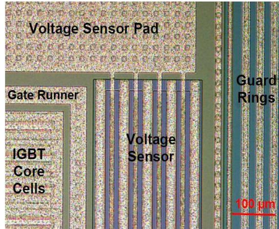
**Fig. 2** Detailed view of the stripped anode voltage sensor and its monolithic integration within the core IGBT
