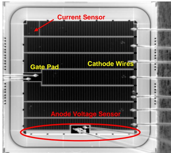
**Fig. 3** Top view of a fabricated 3.3 kV – 50 A IGBT packaged for anode voltage sensor test
