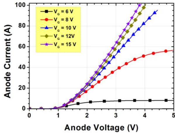
Fig. 5 Experimental I(V) curves of the 3.3 kV IGBT
