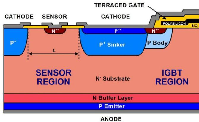
**Fig. 1** Cross-section of the last IGBT core cell and the sensor region
