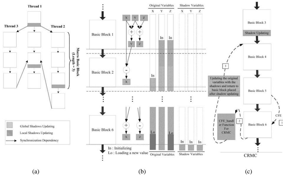
**Fig. 10** CFG and DFG generated from program code ((a): local and global shadows places, (b): local shadow updating, (c): scheme of CRMC)
