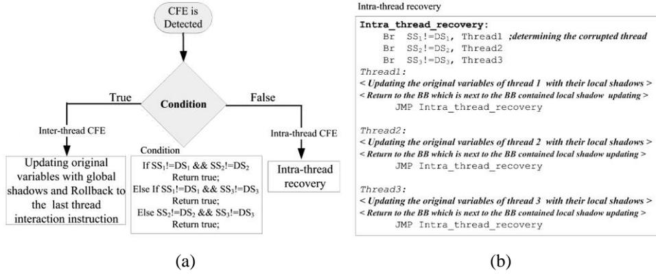
Fig. 11 CRMC scheme ((a): sample flowchart, (b): CFE-handler function)
