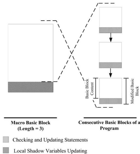
**Fig. 9** Illustration of the shadow variables updating location.
