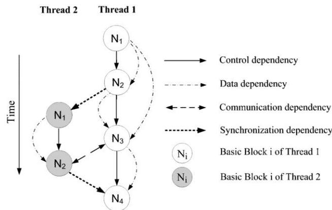
**Fig. 2** Multithreaded program dependency graph.
