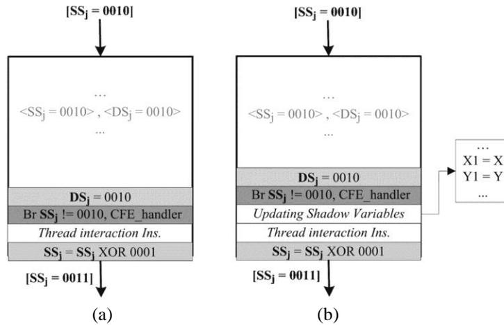
Fig. 3 Illustration of added instructions for methods: (a):CRDC (b):CRMC.
