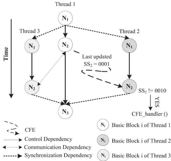
**Fig. 5** Inter-thread CFE detection.
