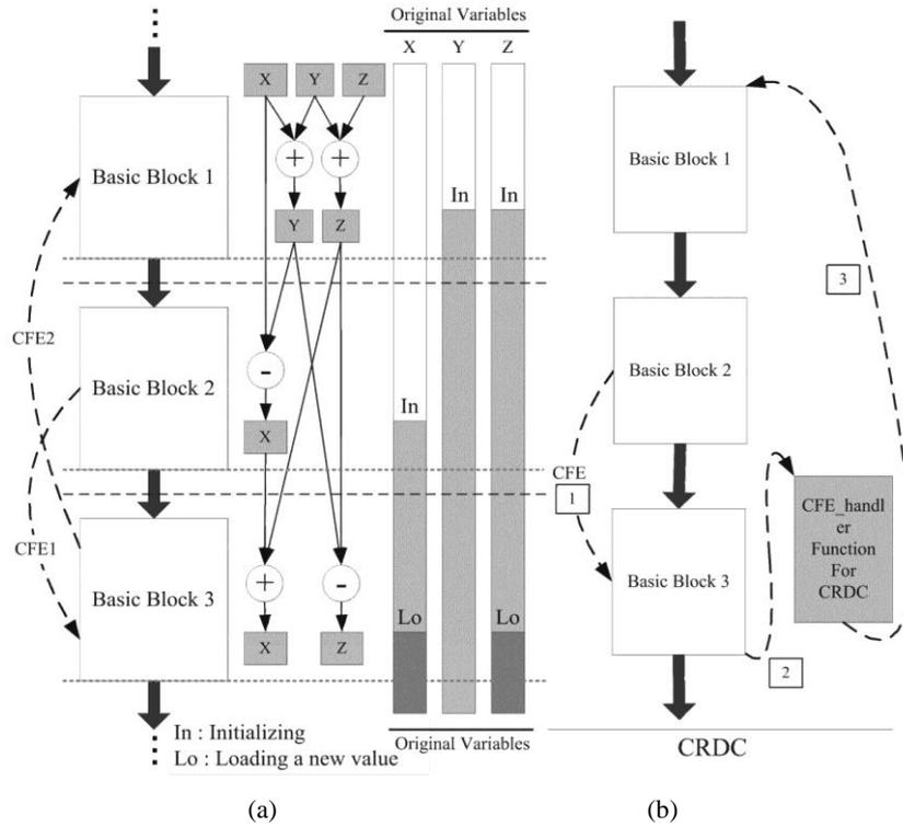
**Fig. 6** (a): CFG and DFG generated from program code, (b): Scheme of CRDC methods
