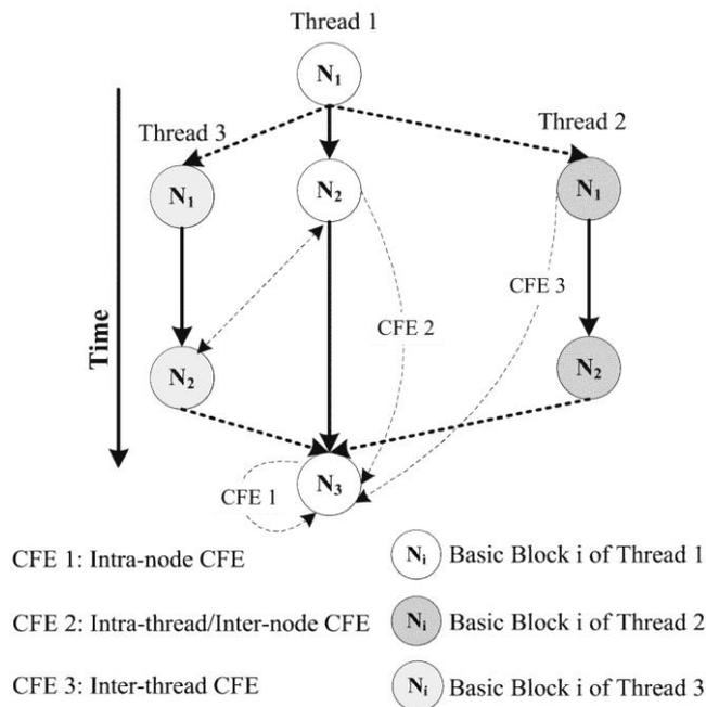
Fig. 4 Illustration of CFE types in CFG scheme.
