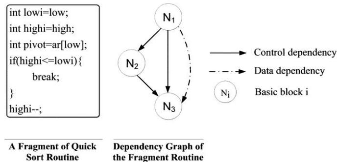
Fig. 1 Single thread dependency graph.
