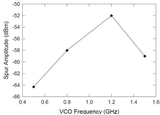
**Fig. 11** Levels of primary spur observed at the VCO's output.
