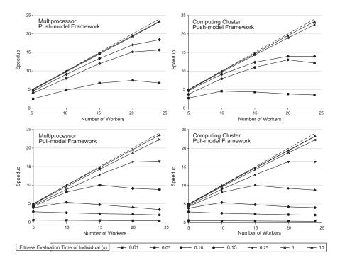
Fig. 3.1: Speedup analysis of the distributed GA run
