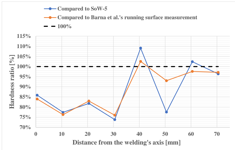
Fig. 14 Surface hardness ratio values of Sample #2 considering the -0.5 mm below the running surface (considering the literature [48,49])
