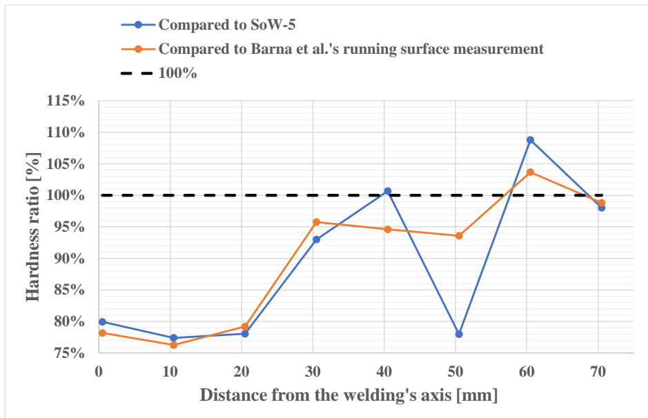
Fig. 15 Surface hardness ratio values of Sample #2 considering the -20.5 mm below the running surface (considering the literature [48,49])
