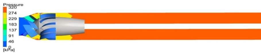
Fig. 16 Pressure distribution in the outlet pipe
