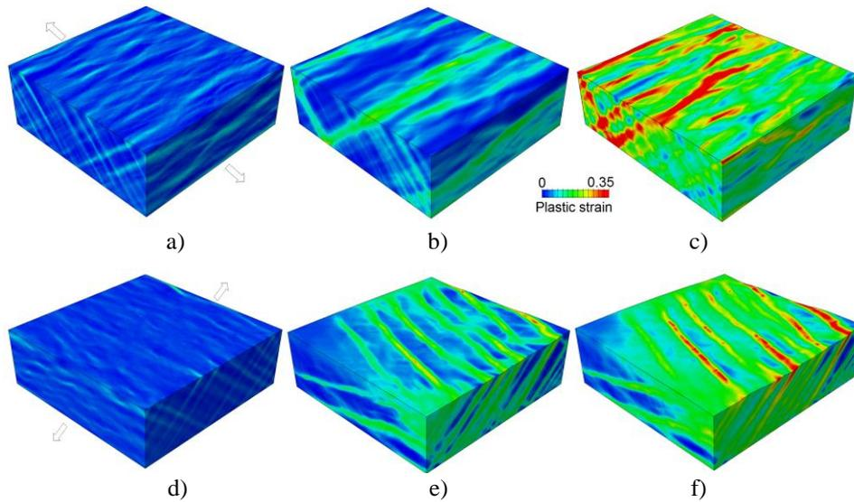
**Fig. 4** Equivalent plastic strains in the textured polycrystal composed of extended grains loaded along the  $X_1$ - (a–c) and  $X_2$ -axes (d–f) at an engineering strain of 0.75% (a and d), 3.5% (b and e) and 7.5% (c and f)
