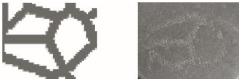
Fig. 14 Designed simple voxel model (left). Fabricated Na-Alginate sample based on voxel model (right) [26]
