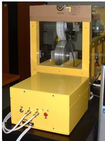
Fig. 2 ABS experimental setup in the Intelligent Control Systems Laboratory of the Politehnica University of Timisoara, Romania [65]
