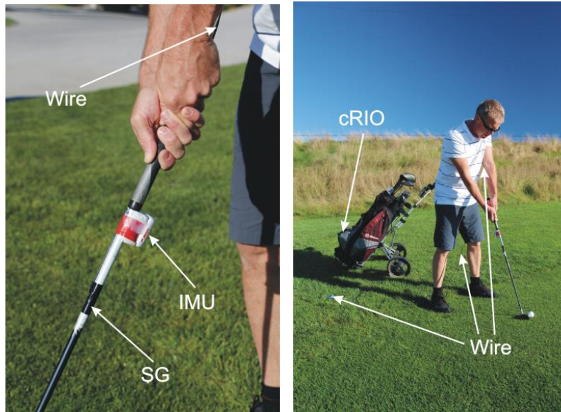
Fig. 3 Smart club prototype used in the field
