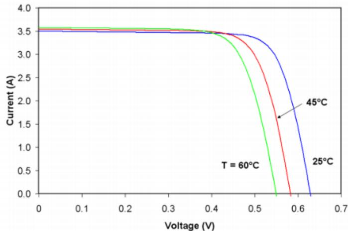
**Fig. 1** The impact of monocrystalline silicon solar cell temperature on its current-voltage characteristic
