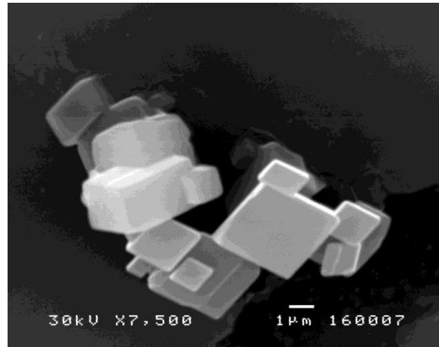
**Fig. 4** SEM image of  $\text{CaCO}_3$  particles at magnification of  $U=7500\times$
