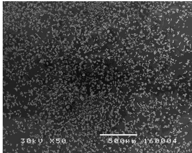
**Fig. 3** SEM image of CaCO<sub>3</sub> particles at magnification of U=50×
