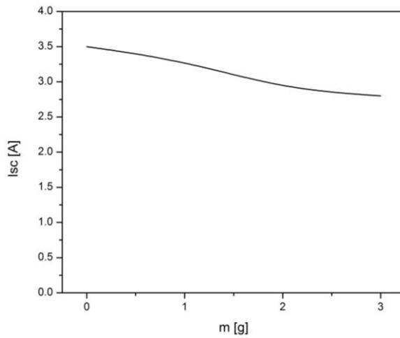
**Fig. 6** Dependence of  $I_{sc}$  on the horizontally mounted solar module surface soiling with different amounts of  $\text{CaCO}_3$
