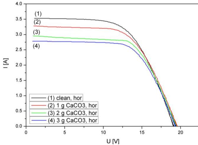
**Fig. 5** Current-voltage characteristics of the horizontally mounted solar module depending on the soiling of its surface with different amounts of  $\text{CaCO}_3$
