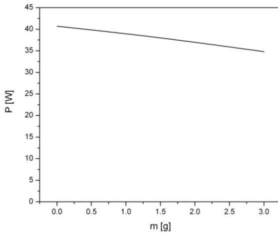
**Fig. 8** Dependence of the power obtained by horizontally mounted solar modules on the soiling of their surfaces with different amounts of  $\text{CaCO}_3$
