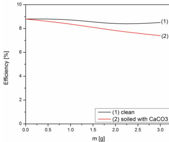
**Fig. 10** The dependence of the efficiency of a horizontally mounted clean and solar module soiled with  $\text{CaCO}_3$
