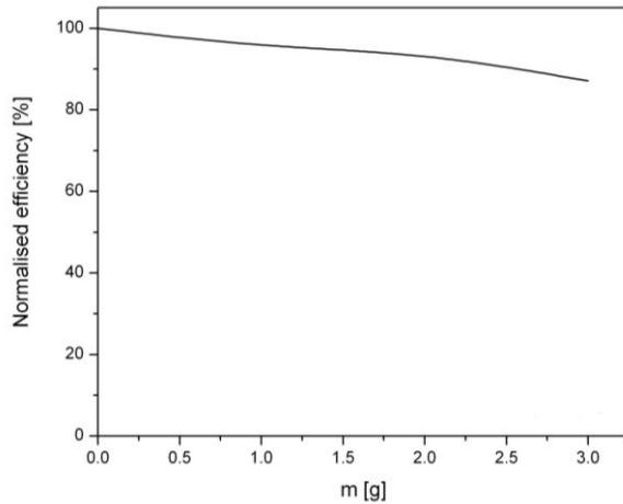
**Fig. 11** Dependence of the normalized efficiency of a horizontally mounted solar module on the soiling of its surface with different amounts of  $\text{CaCO}_3$
