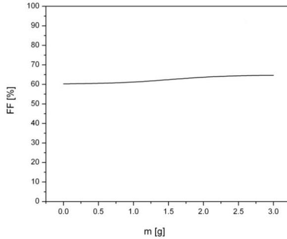
**Fig. 9**  $FF$  dependence on the the horizontally mounted solar module surface soiling with different amounts of  $\text{CaCO}_3$
