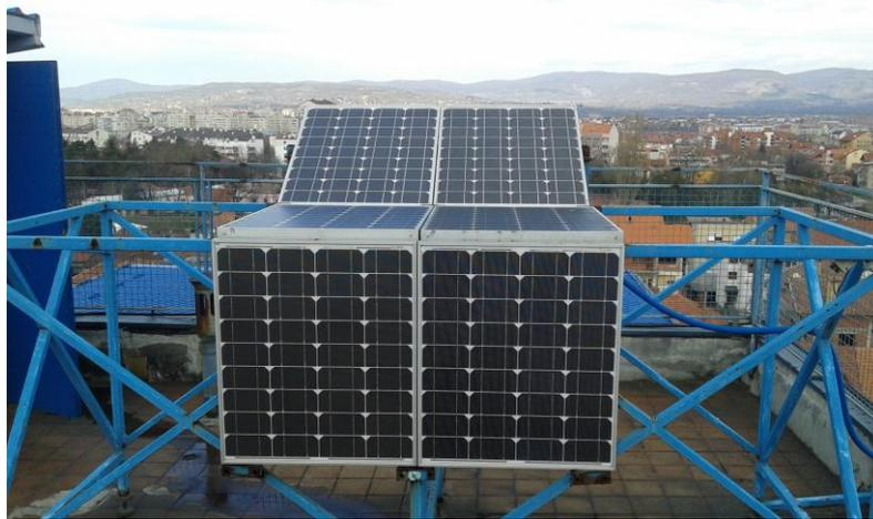
**Fig. 2** A system of two identical solar modules ISF-60/12, each of individual power of 60 Wp, horizontally mounted, southward facing
