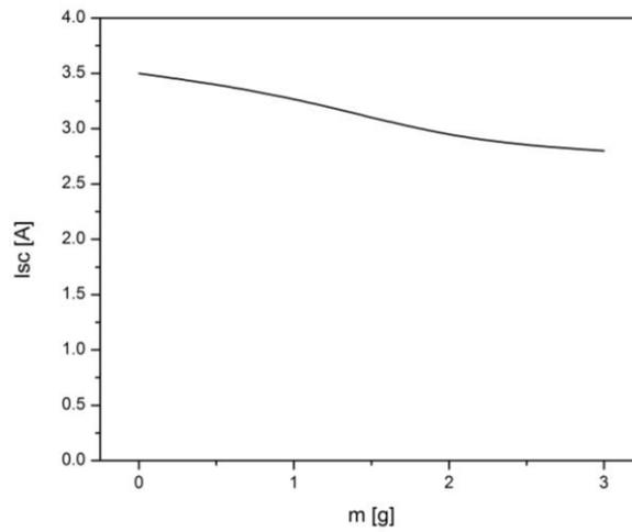
**Fig. 6** Dependence of  $I_{sc}$  on the horizontally mounted solar module surface soiling with different amounts of CaCO<sub>3</sub>
