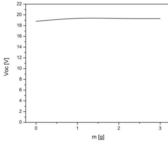
**Fig. 7** Dependence of  $U_{oc}$  on the horizontally mounted solar module surface soiling with different amounts of  $\text{CaCO}_3$
