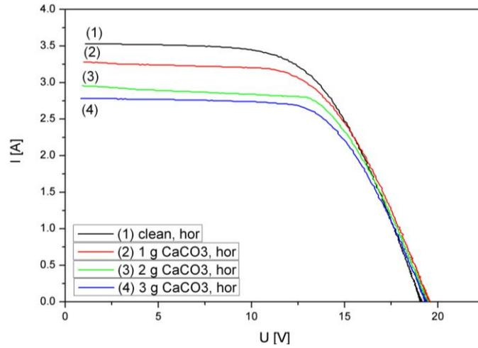
**Fig. 5** Current-voltage characteristics of the horizontally mounted solar module depending on the soiling of its surface with different amounts of CaCO<sub>3</sub>
