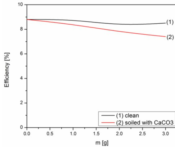
**Fig. 10** The dependence of the efficiency of a horizontally mounted clean and solar module soiled with  $\text{CaCO}_3$
