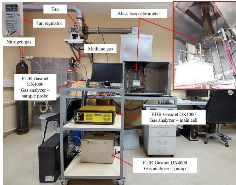
**Fig. 1** Custom made assembly: mass loss calorimeter, extraction fume hood assembly, and FTIR gas analysis system
