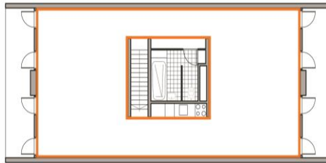
Fig. 2 The principle of stratification with designated “frame and generic space”
