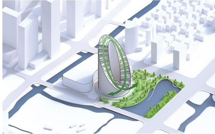
Fig. 7 Daylight, minimize outward facing surface area of more solar exposed facades. (Source: https://www.archdaily.com )
