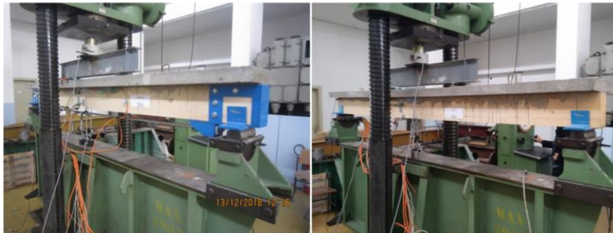
Fig. 9 Girders prepared for testing
