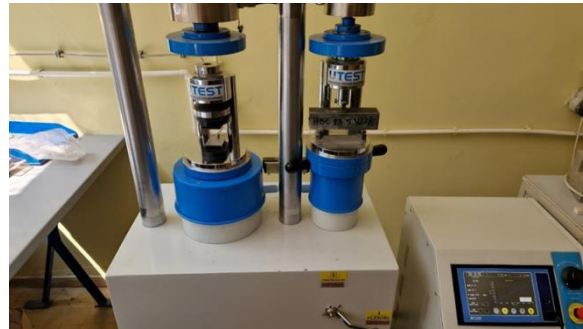
Fig. 2 Test setup for flexural strength testing
