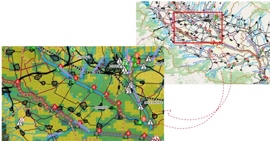
Fig. 2 Case study area as produced within the QGIS environment and zoom in regions with numerous flood protection works (e.g. red triangles and green squares attributes the works of the removal of deposits, and cleaning of bridges' piers from sediments).
