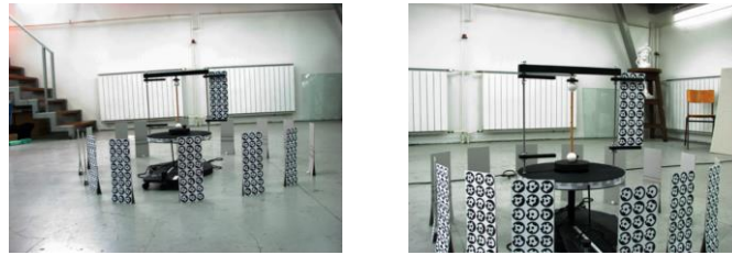
Fig. 1 Artificial experimental scene (Referral Test-Field): centrally positioned equipment used to fix vertically the experimental linear object; “RAD” target panels distributed radially in its surrounding
