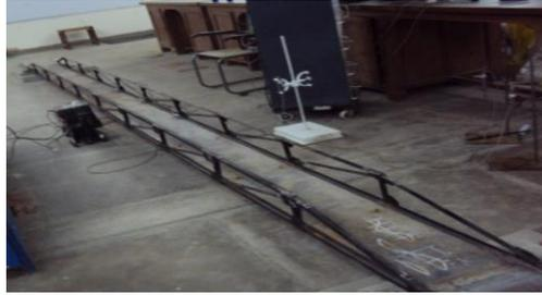
**Fig. 1** Lab Model for through type Steel Bridge
