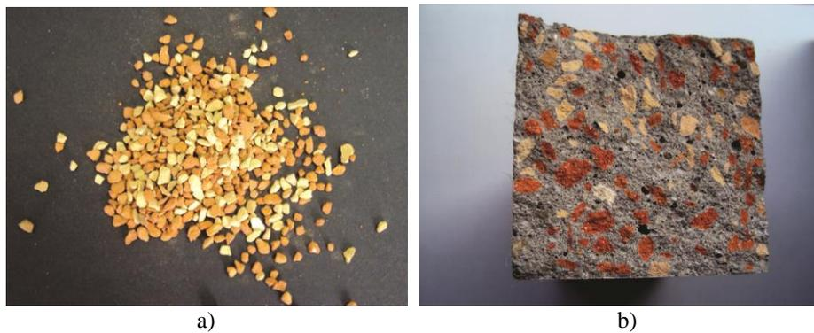
**Fig. 1** Used materials: a) recycled crushed brick aggregate 2/4 mm,
