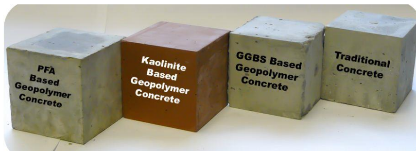
Fig. 1 Range of geopolymer-concrete and ordinary-concrete [6].
