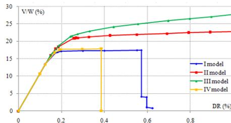
**Fig. 1** Developed NSPA pushover curves for all analyzed models of mechanisms
