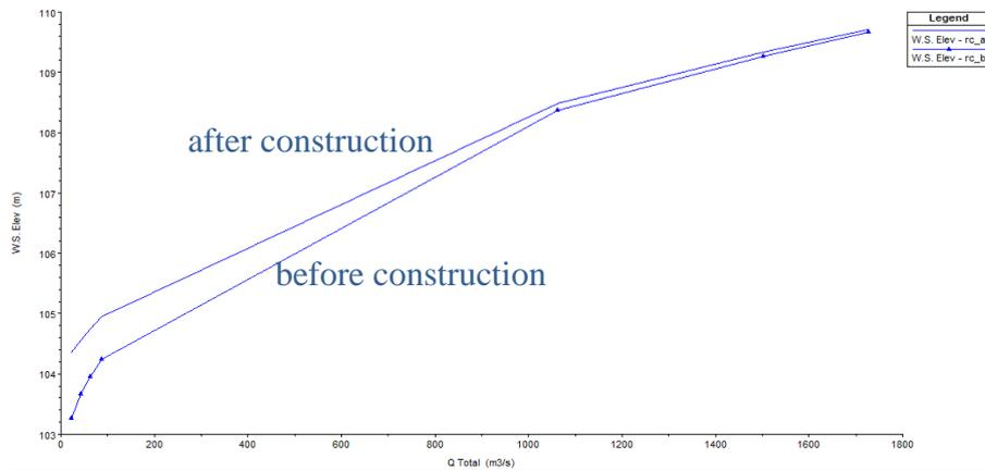
**Fig. 7** Rating curves before and after construction
