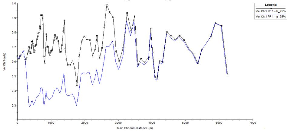
Fig. 6A Flow velocity curves before and after construction for  $Q_{25\%}$
