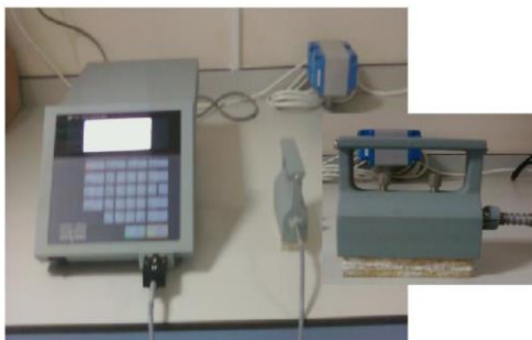
Fig. 4. The experimental setup for measuring thermal conductivity coefficient
