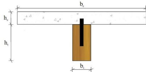
**Fig. 1** Timber-concrete composite cross section
