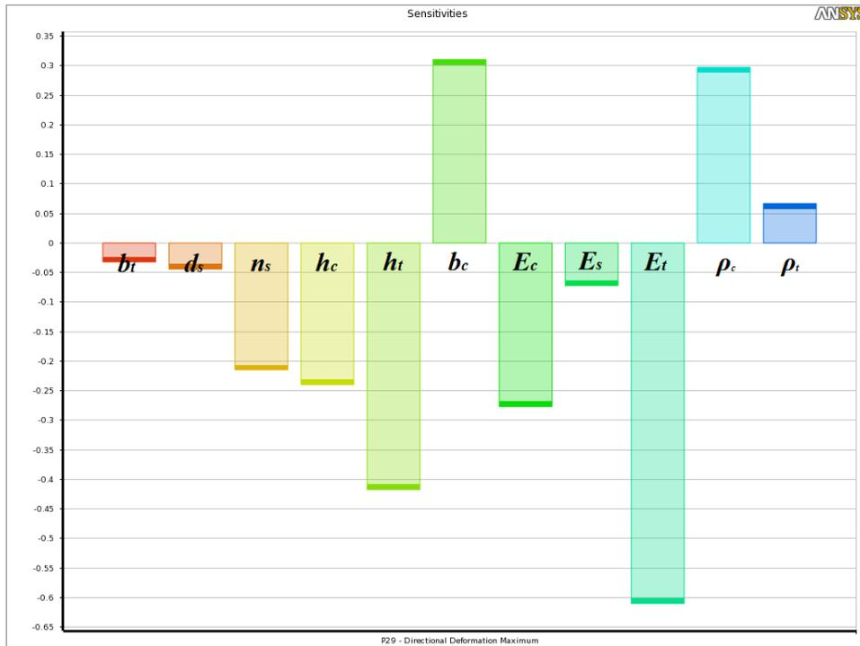
**Fig. 4** Sensitivities of the maximum mid-span deflection
