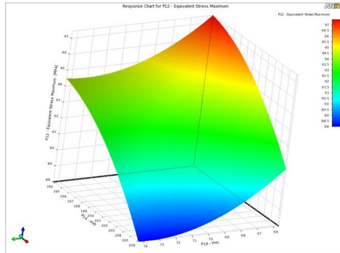
**Fig. 5** Response surface for maximum equivalent stress
