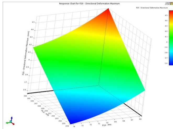
**Fig. 6** Response surface for maximum mid-span deflection
