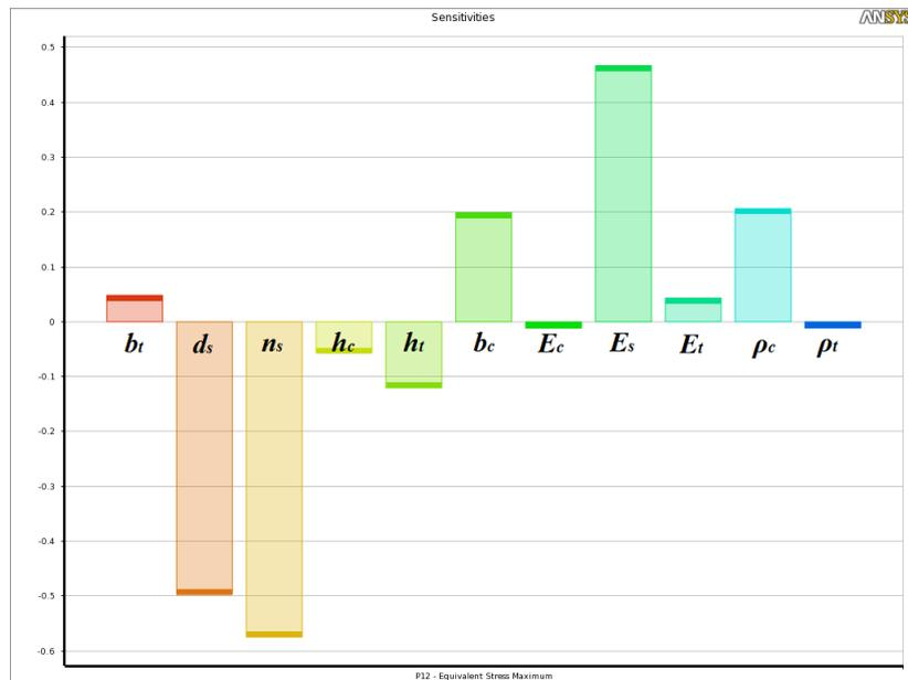
**Fig. 3** Sensitivities of the maximum equivalent stress
