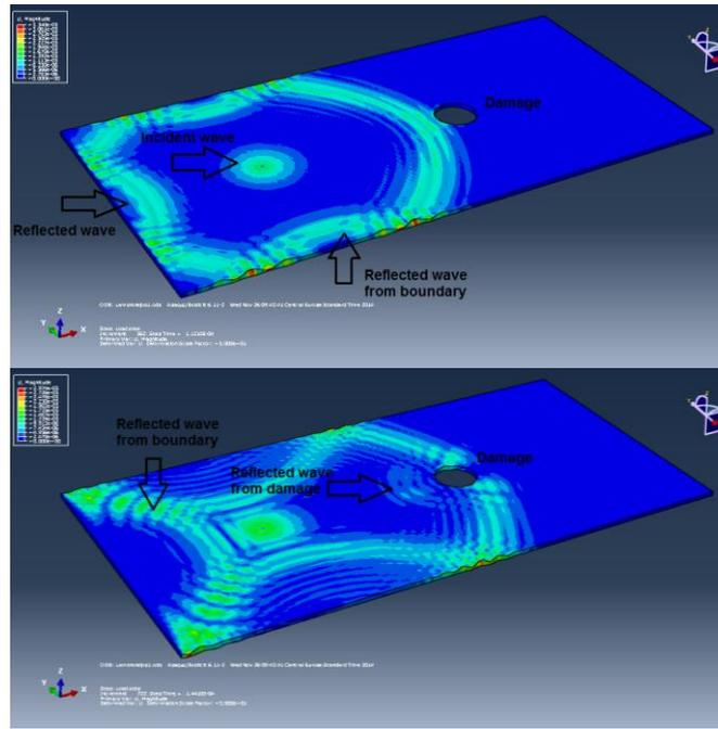
**Fig. 6** Lamb wave propagation at steel plates at time points:  $11.21 \text{ e}^{-5}(\text{s})$  and  $14.43 \text{ e}^{-5}(\text{s})$ .
