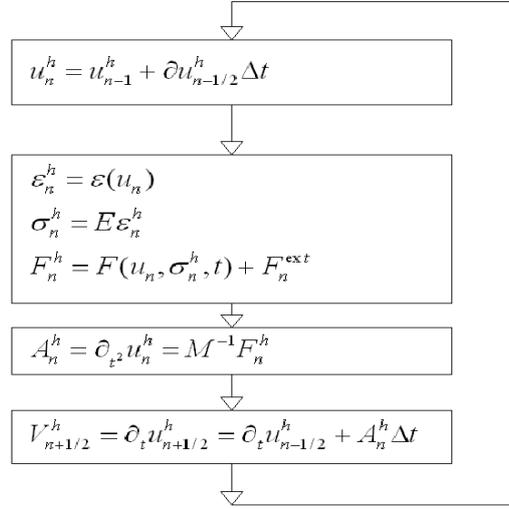
Fig. 1 Procedure of explicit finite element method
