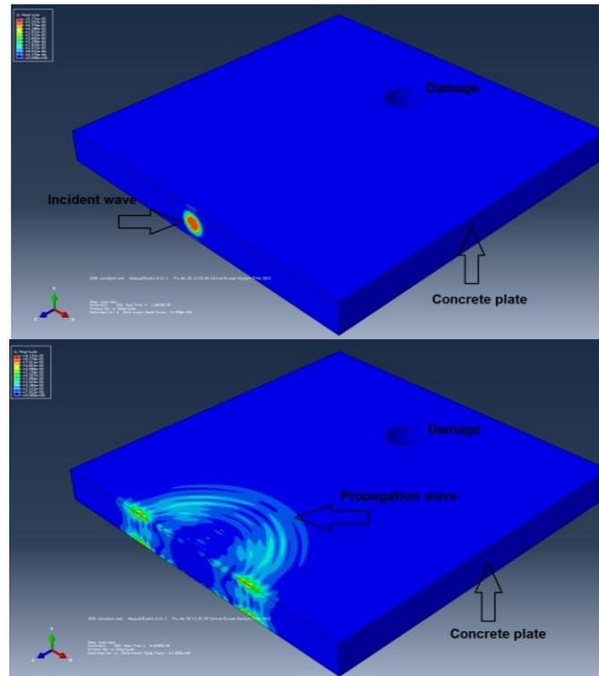
**Fig. 3** Wave propagation at concrete plates at time points:  $1.06 \cdot 10^{-5}$  (s) and  $6.65 \cdot 10^{-5}$  (s).
