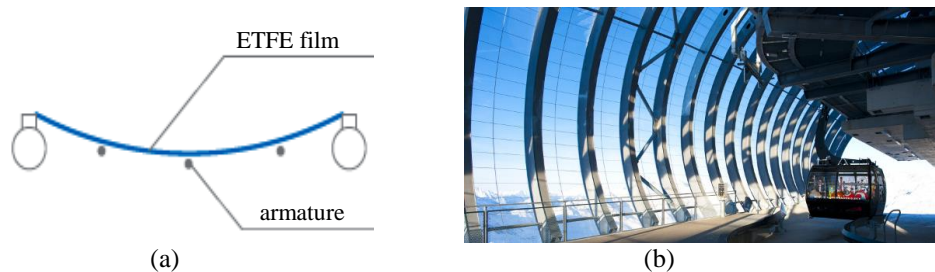
Fig. 5 a) Cross section of single layer ETFE film panel; b) Gaislachkogel gondola [17];
