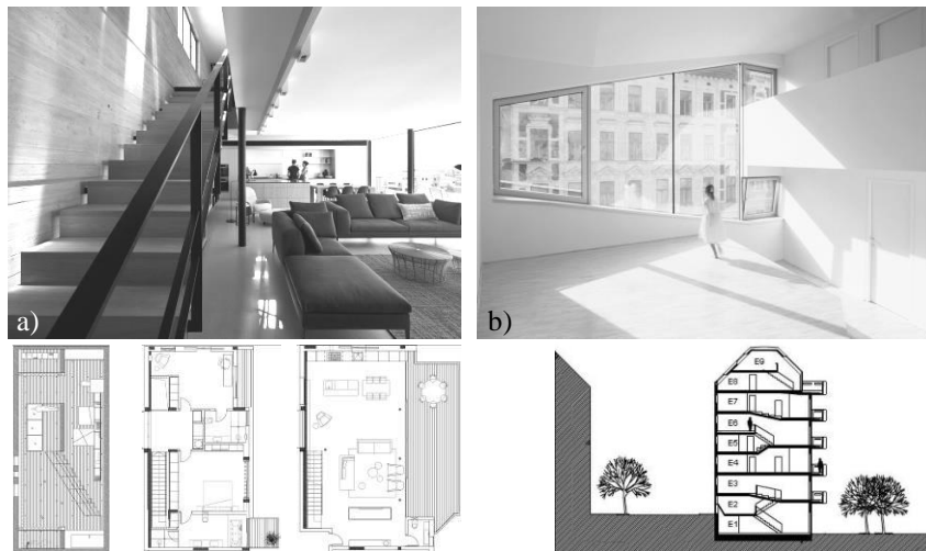
Fig. 10 a) Duplex apartment with day and night zones separated on different floors; b) apartment designed with split-levels and increased ceiling heights of certain rooms
