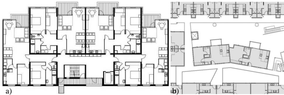
Fig. 6 a) Separation of groups of several apartments from vertical circulation space, forming a semi-private space in front of their entrances; b) withdrawal of the entrances from horizontal circulation space
