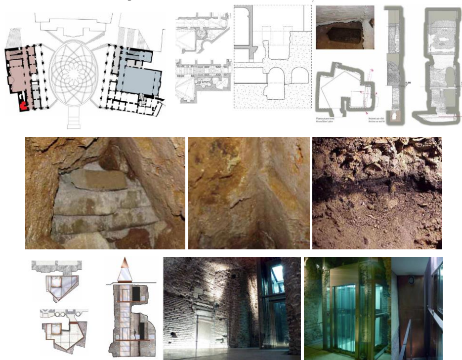
Fig. 8 The elevator the Capitoline Museum - Campidoglio in Rome: the situation, the location of the elevator, photo during construction, base and cross section, layers of the ground, layout drawings and outcome [2].
