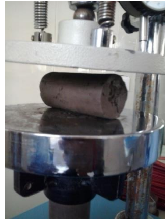
Fig. 6 Splitting tensile strength test set up
