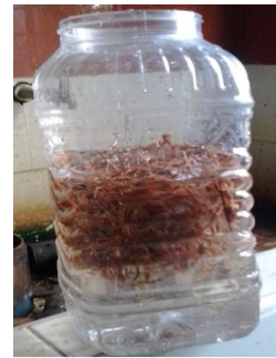
Fig. 2 Water absorption tests on coir fiber
