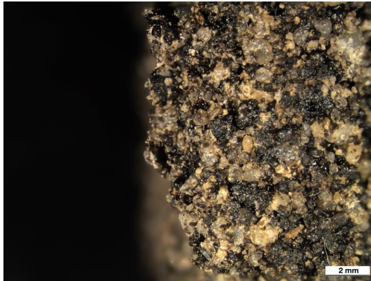
Fig. 9 Photograph of a broken edge of the specimen after testing
