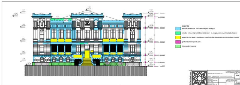
Fig. 4 "Karadžorđev dom", main façade (northeast) deterioration mapping, author: E.V.Petrović (November 2020)
