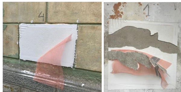
Fig. 6 “Karađorđev dom”, “pull-off” test results (test No4)-left, test results (test No1)-right, author: E.V.Petrović (November 2020)
