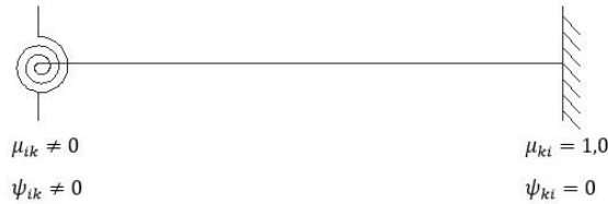
Fig. 7 Semi rigid connection at left node and ideally rigid connection at right node
