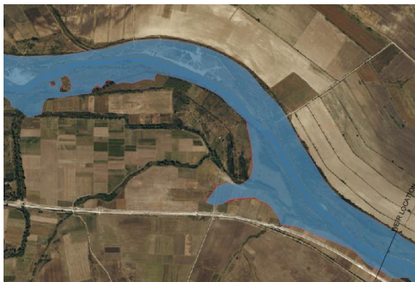
Fig. 8C Flooded areas at Q_{1\%}
