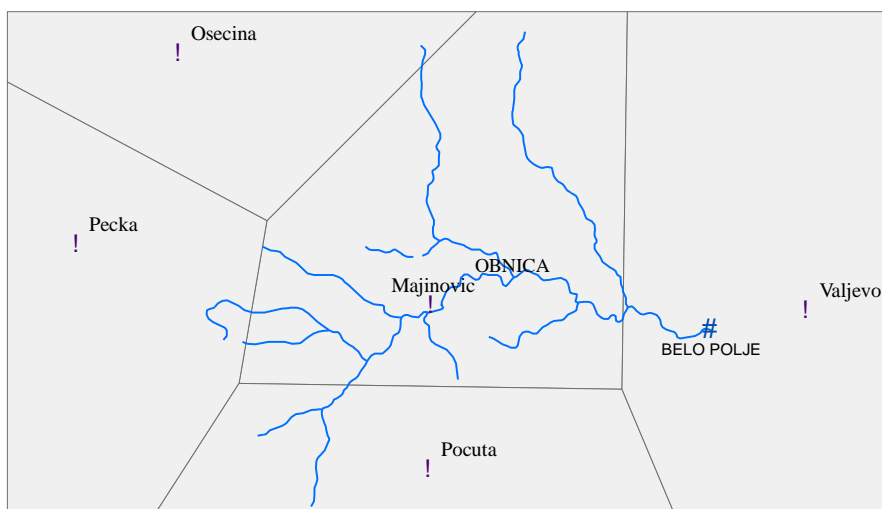
Fig. 2 The Obnica River basin with hydrological station (blue triangle), rain gauges (violet dots) and Thiessen polygons for the rain gauges
